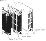
To identify the style of a radiator, count the number of tubes or columns. Then, check the width. When you have identified the style (1, 2, or 3) read the radiation per section beneath the radiator style.
